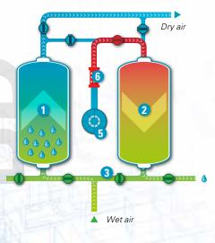
The blower (5) takes ambient air and blows it over the external heater (6). The heated air is then sent through the saturated desiccant (2), forcing the adsorbed moisture out, from top to bottom.
