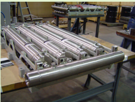
Low pressure, SS dryers, 400 SCFM
