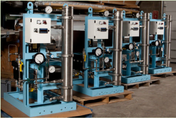
Dryer & instrumentation package, 750 PSIG Design
