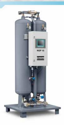
Atlas Copco's new nitrogen generator uses Pressure Swing Adsorption technology to isolate nitrogen molecules from other molecules in compressed air. Oxygen,  $CO_2$ , water vapor and other gasses are adsorbed. The result is virtually pure nitrogen at the outlet of the generator. The NGP series are a very cost-efficient source of nitrogen used in various industries like food and beverage, metal processing, electronics, and many others.
