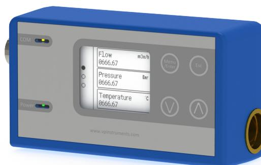
The VPFlowScope In-line 3/8" measures flow, total flow and temperature. Thanks to the patented Thermabridge™ technology, the VPFlowScope In-line can perform bi-directional flow measurements. The built-in display will show the actual and total flow, and the Modbus and analog 4 .. 20 mA outputs enable you to interface with VPVision or other monitoring systems.
