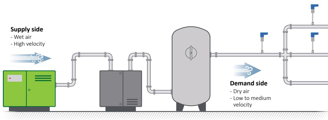
*Measure dry and clean gas only for correct measurements and a long lifetime.*
