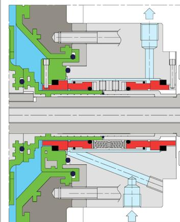
Applications where no leakage to atmosphere can be tolerated e.g. hazardous, toxic, inflammable media.
